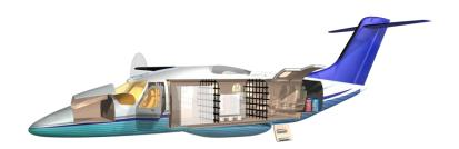
Time for interior change from all passenger version to combi version in less than 30 minutes
